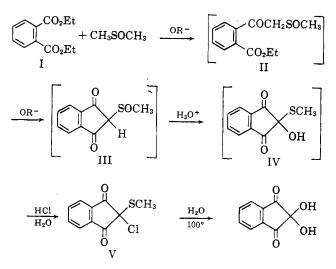
The condensation occurs upon the addition of diethyl phthalate to a solution (or suspension) of an alkali metal alkoxide in anhydrous dimethyl sulfoxide under an atmosphere of dry, oxygen-free nitrogen. Removal of the solvent by vacuum distillation leaves a salt (presumably the alkali metal salt of III) which is soluble in water. When the aqueous solution of this salt is added to 5 Mhydrochloric acid V rapidly precipitates in a high state of purity.
